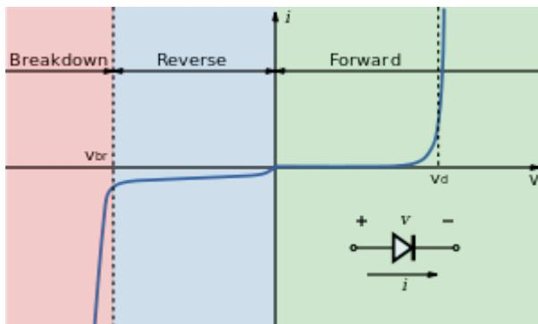
I-V diagram for a LED resembles I-V diagram for a diode. An LED will begin to emit light when the on-voltage is exceeded. Typical on-voltages are 1...2 V for infrared LEDs, 2...4 volts for visible LEDs and more than 4 V for UV LEDs.
