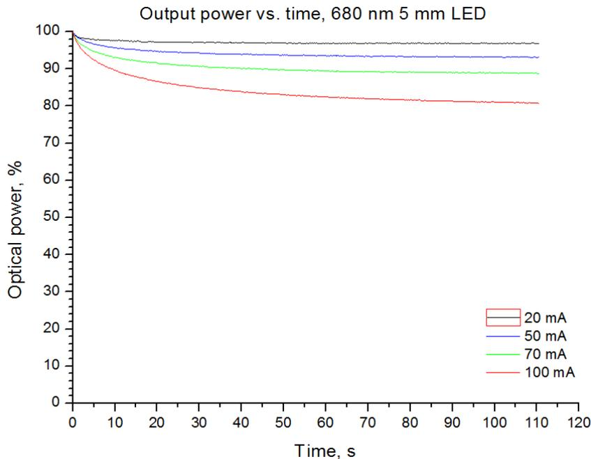
Figure: Output power stabilization of a 680 nm deep red LED at different currents.
