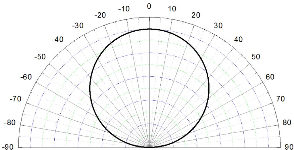
$\pm 60$  (120) degrees LED. Lambertian distribution is typical for many chips and SMD LEDs.
