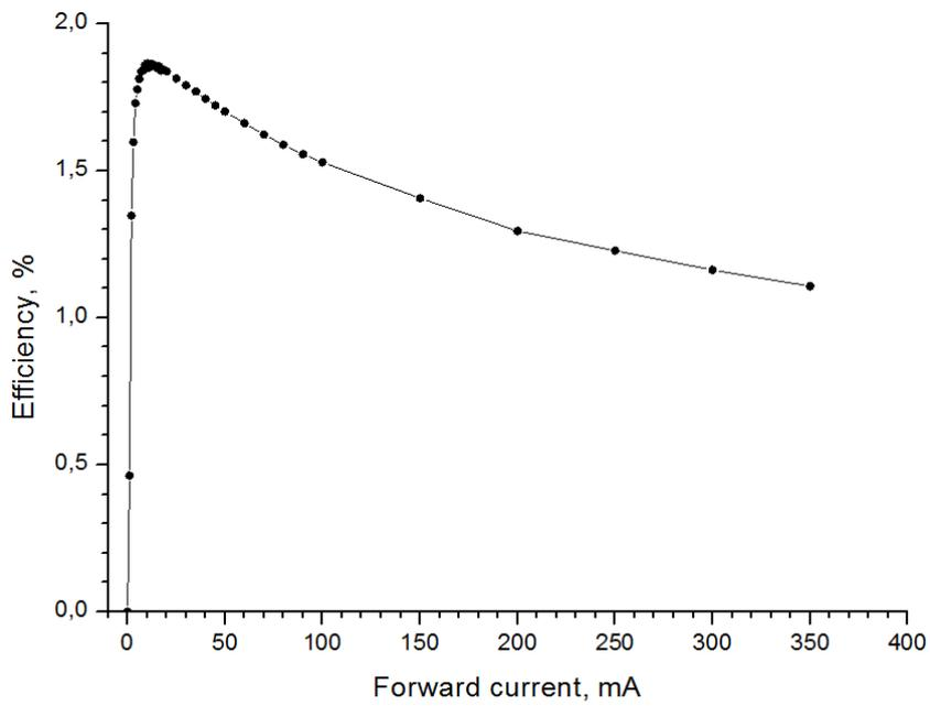
Figure. Energy conversion efficiency vs. current, Nikkiso 285 nm SMD 3535 UV LED.
