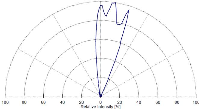
figure: This is a radiation pattern of 3 mm visible LED shows a profound difference between optical and mechanical axis.
