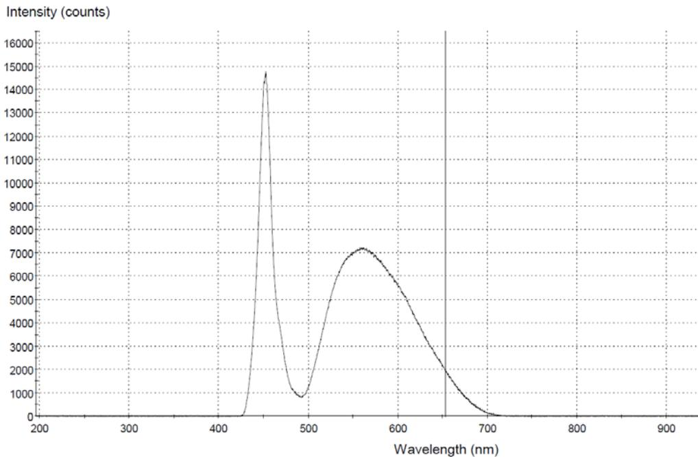
Figure: spectrum of a single-chip white LED.
