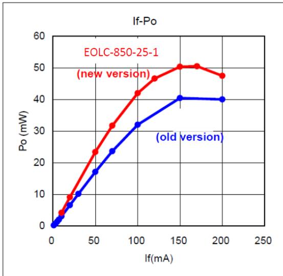
\*LED die was mounted on TO-18 header without resin coat.
