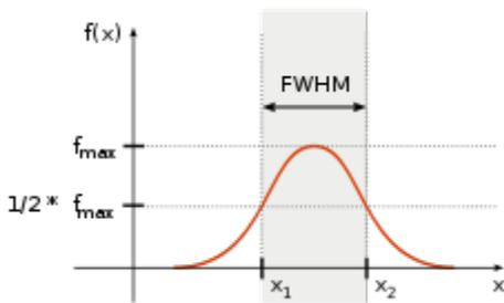
typical spectral widths (FWHM) of LEDs, usually increasing with increasing peak wavelength ( $\Delta\lambda_{0.5}$  is about 5% of  $\lambda_P$ )
